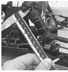
**Step 3:** Measure from the center of the shock standoff screw to the center of the shock riser button to get your final droop setting. The front shocks should both be set at the same lenght, as should the rear shocks. \* The normal droop setting is between O-5mm from the FULL DROOP measurement.
